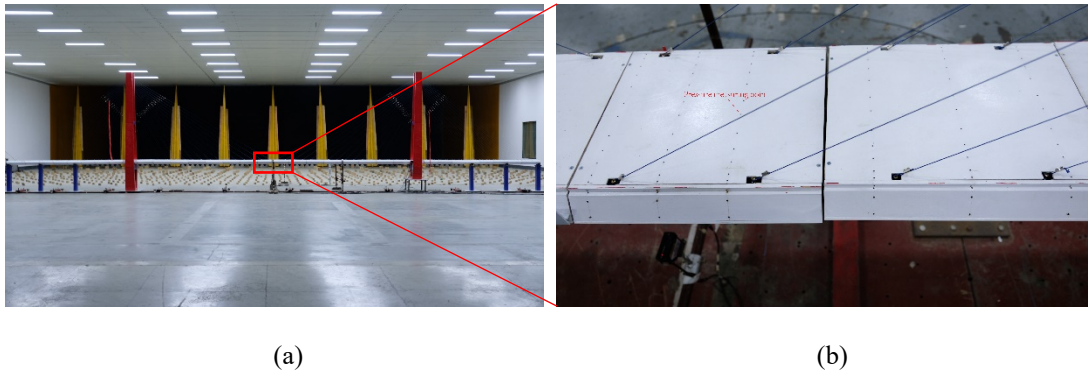
Figure 2. Arrangements for the aeroelastic model (a) aeroelastic model (b) pressure measuring points.
